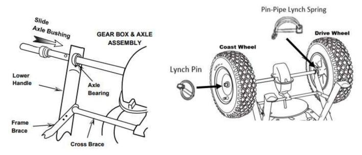
**STEP 5:** Flip spreader over to rest on its tires and stand. Install handle shaft to lower handles and pivot bracket using the 2 inch bolts and locknuts. **Tighten these down now.**
