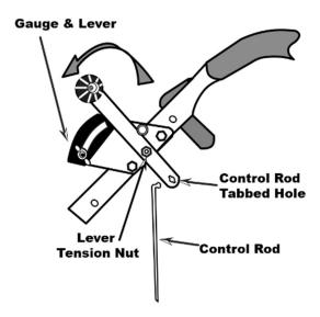
**Step 7:** Push lever all the way forward to full OPEN setting. Align and push the threaded end of the Control Rod through the 'L' bracket. Your handle lever should now be pushed back to the CLOSED position on the gauge. Now, adjust both nuts so that the 'L' bracket sits firmly between the two nuts. Move the top nut first then the bottom.
