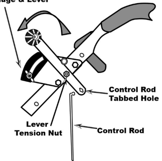
**STEP 2:** Install CONTROL ROD into handle as shown above. TIP: Install the CONTROL ROD using pliers to squeeze into LEVER.
