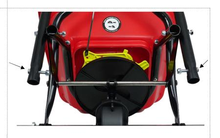
**Step 3:** Rotate the DRAW BAR down and attach the DRAW BAR to the FRAME BRACES with the two bolts you just removed.
